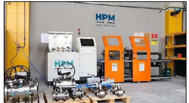
Pressure & Func. Test Benches Advanced SCADA enabled Pressure test bench.
