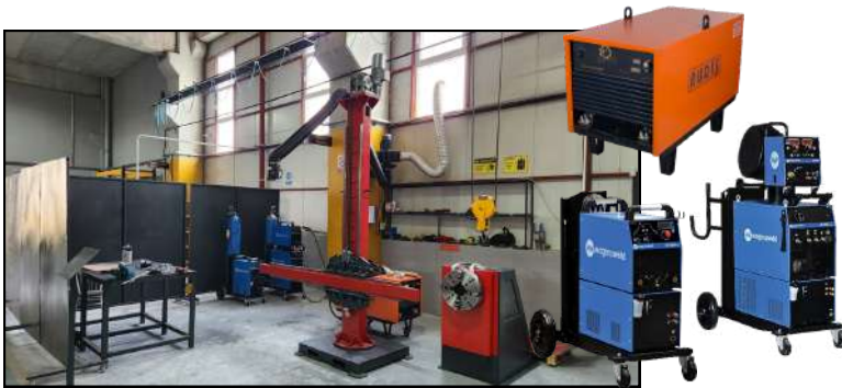
In-house Semi-Automatic GTAW (TIG), MIG and SAW with Welding positioner facility from 1 mm wall thickness.
